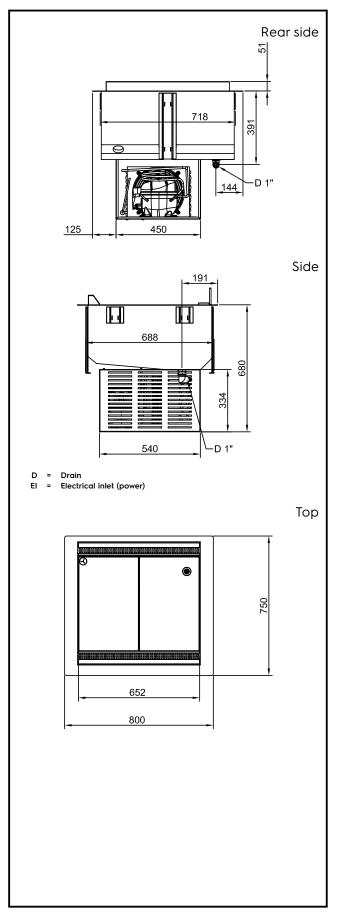
Drop-In Drop-in refrigerated well, ventilated (2 GN container capacity)
