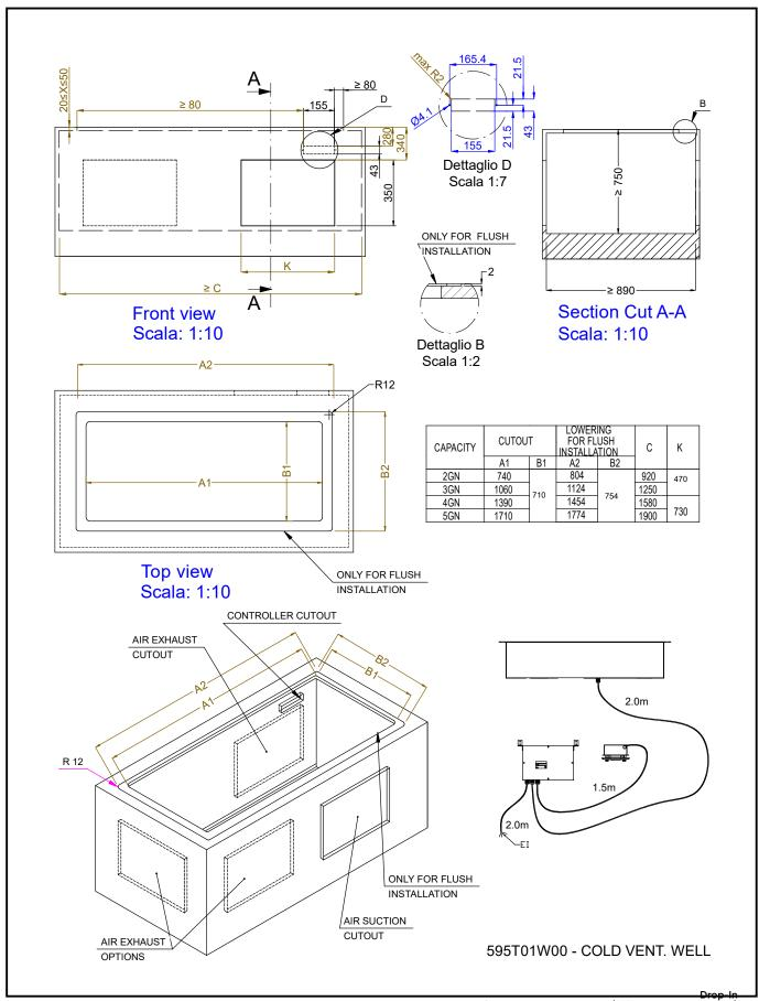
Drop-in refrigerated well, ventilated (2 GN container capacity)
